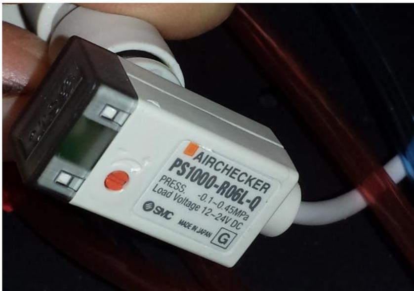
The Orange coloured adjustment screw will be covered by a security label when factory set.
