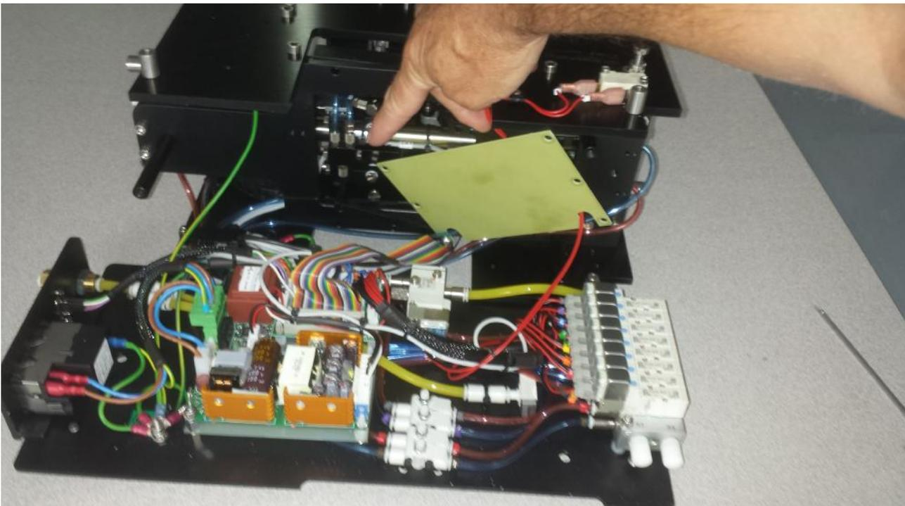
There is an pneumatic fitting assembly here with blanking screws, check here to ensure no air leak present in this area.
