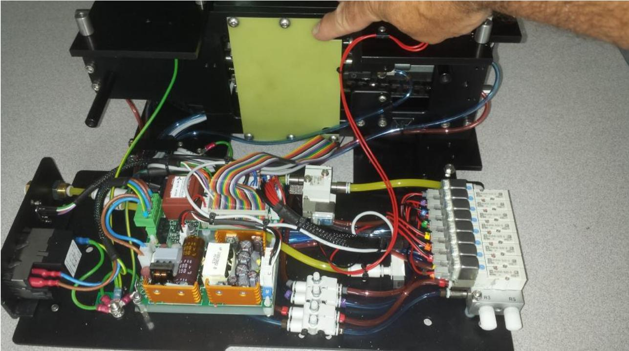
Remove this panel to access air fitting behind, Be careful do not lose the spacer bar fitted!
