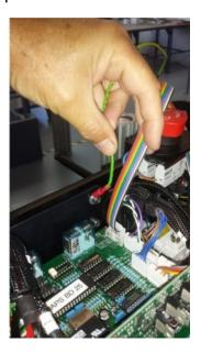
6. After removal of touch screen and protective earth connections, continue to lift cover vertically to fully remove cover from KAPs chassis.
