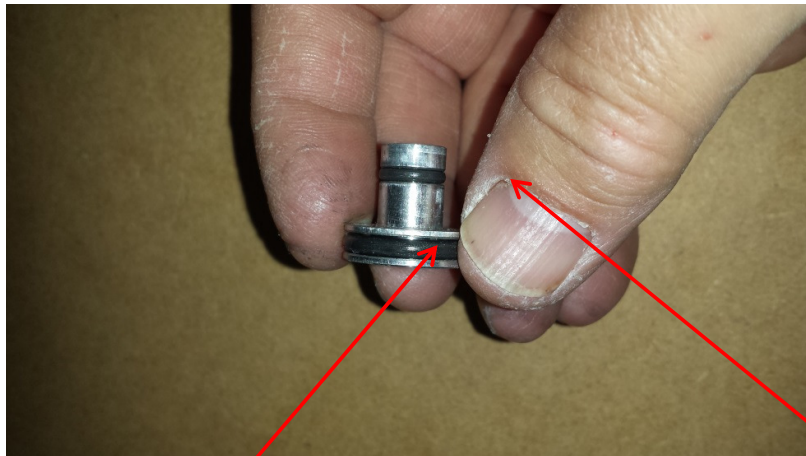
Sealing O ring Part number. 3032-10003
