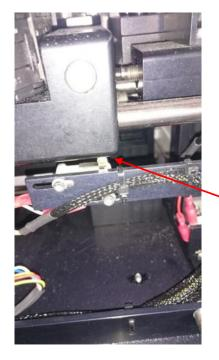
Both Front and Rear switches are activated by the shuttle axis as shown
