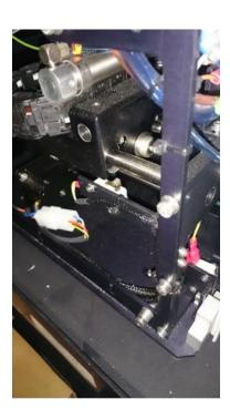
The shuttle unit carriage will activate this switch, it also time sensitive, so if the air pressure is low or the shuttle is traveling too slowly then the time taken to activate the switch can also cause a 'time out' error, the timer is hard coded into the software so cannot be adjusted.
